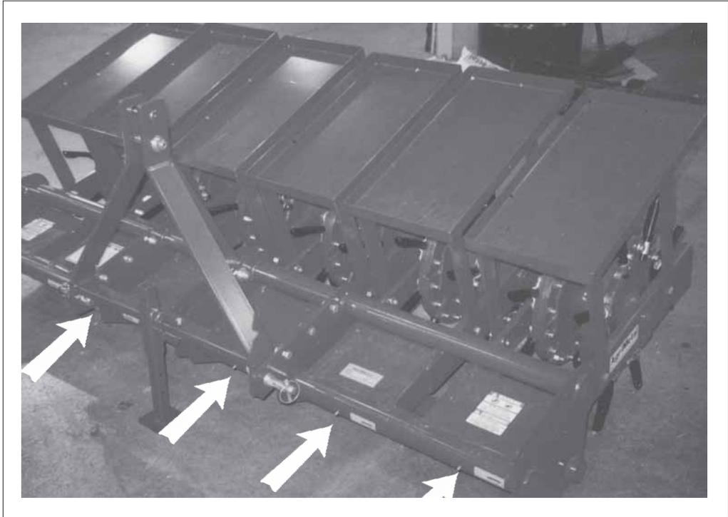
Fig. 22 AERATING WHEEL PIVOT SHAFT
