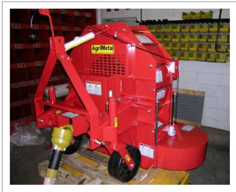
**Fig. 13 3 POINT HITCH AND PTO**
