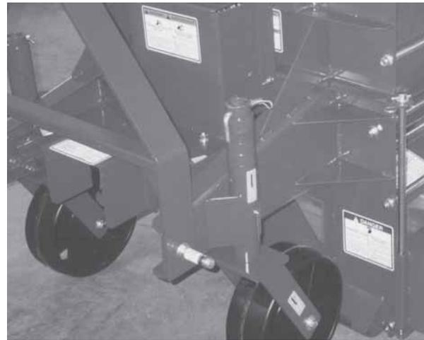
Fig. 27 GAUGE WHEEL ADJUSTMENT
