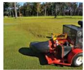
◆ THE TB-380 I.C. IS MOUNTED LOW TO RELEASE THE AIR STREAM HORIZONTALLY AT GROUND LEVEL. THIS, RESULTS IN THE MOST PERFORMANT TURBINE ON THE MARKET. A FULL LENGTH SKID PLATE IS MOUNTED BENEATH THE FRAME TO ELIMINATE ANY RISK OF SCUFFING. WHETHER YOU BLOW LEAVES, CLIPPINGS OR THATCH; THE TB-380 I.C. WILL CLEAN FAIRWAYS TWICE FASTER THAN ANY OTHER EXISTING TURBINE ON THE MARKET.
