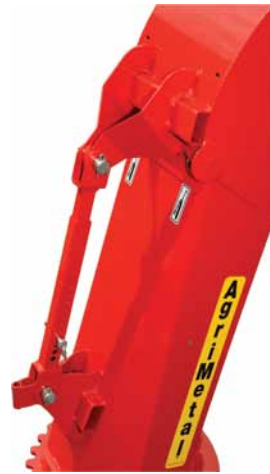
Manual telescopic adjuster for snow chute
