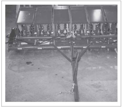
tines. This process is repeated again and again as long as you are moving with the tractor. With the knives, they slice the turf as the wheels turn. This continuous rotation insures an efficient and even aeration of your soils.
