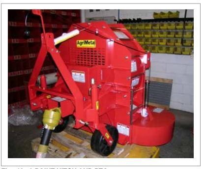
Fig. 13 3 POINT HITCH AND PTO
