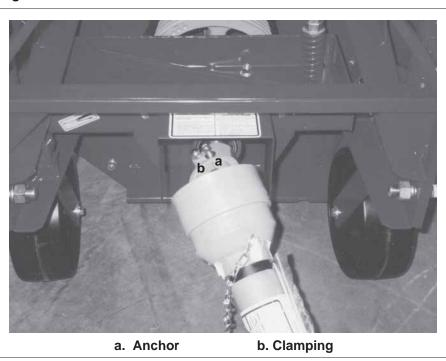
Fig. 9 ANCHOR BOLT
