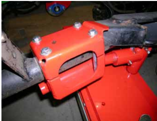
Fig. 2 FRONT ROLLERS RETAINERS
