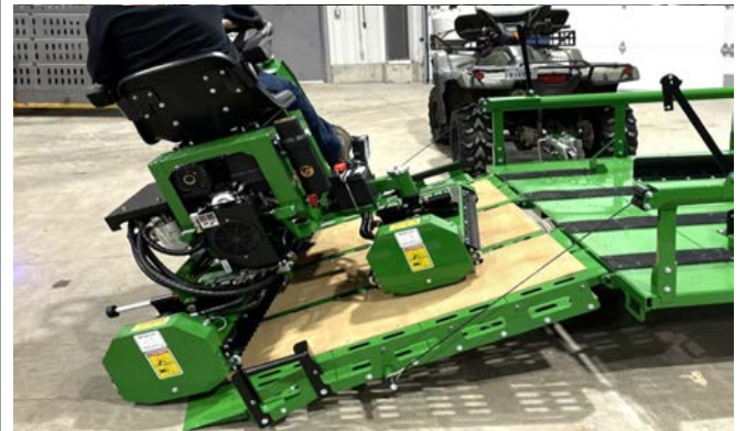
Drive Down Ramp
