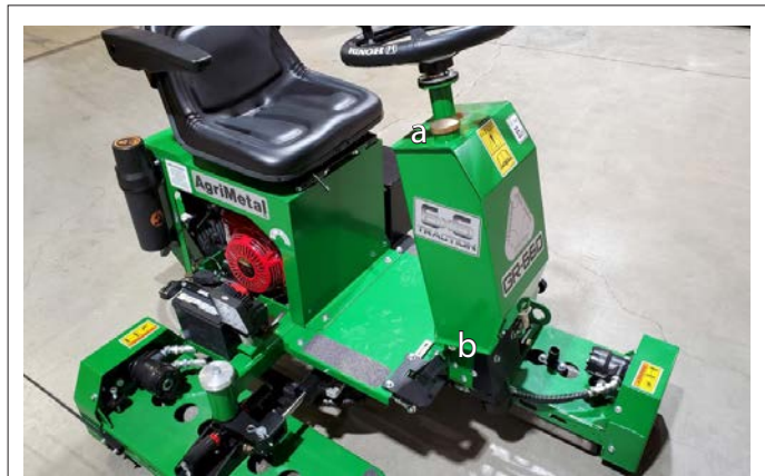
a. Fill/Dipstick b. Drain Plug
